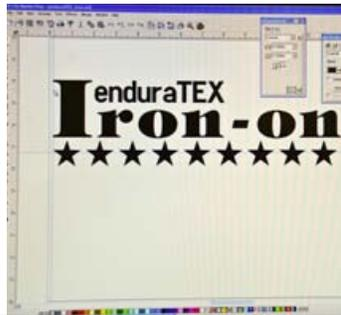
**Step 2:** Before sending the job to the vinyl cutter, flip the graphic to mirror image of original design. You may also have the option of setting this in the control panel of the vinyl cutter.
