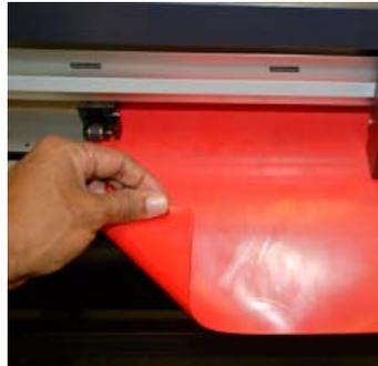
**Step 4:** Set the cutting force for approximately 70 grams or the amount you would use to cut 2 mil cast vinyl. Use a 45° blade. Perform a test cut to ensure that the parameters are correct.
