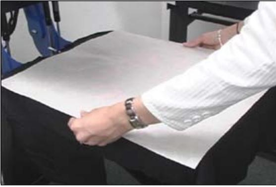
**5** On your heat press, verify that your temperature is set between 300° and 340° F. If your heat press has a built in timer, set it for 15-20 seconds. Place the weeded graphic onto the cotton, polyester, or acrylic fabric with the release liner facing upward. Place the Teflon sheet over the graphic, then close the heat press. After 15-20 seconds, open the press.
