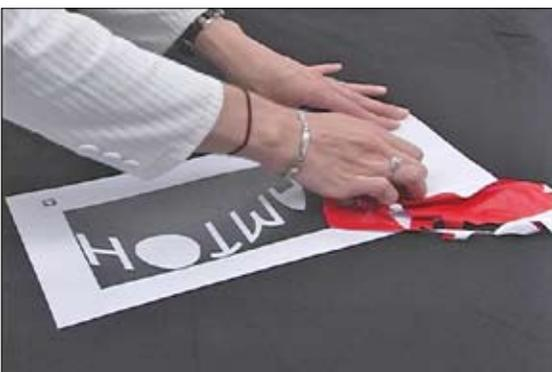
**4** Your plotter will cut a mirror image of the original design into the garment film. When the cut-job is complete, advance the material forward and remove from the cutter using the Xacto, Olfa, or other utility or hobby knife. Using your preferred weeding tool, weed the excess material from the release liner.
