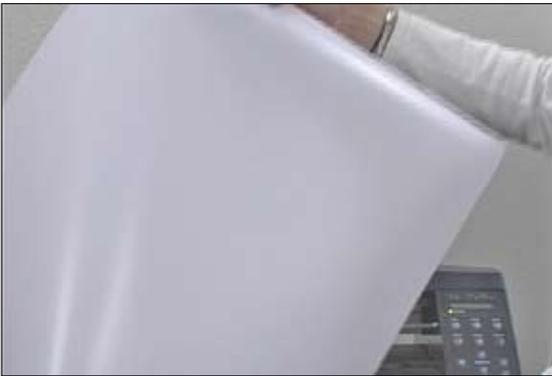
**1** When using EnduraTEX Hotmark 70, you will notice that the release liner is completely white. When you cut, load the colored side downwards into your cutter, allowing the white backing to be facing upwards.
