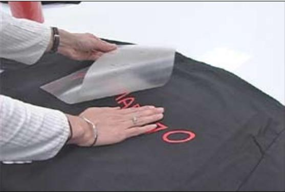
**6** Allow the garment to cool to room temperature before removing the release liner. During this time you may remove the garment from the heat press and place in a location out of the way to allow for a second shirt pressing if desired. After the application has cooled, slowly peel the release liner away from the shirt. The garment film should remain on the fabric resulting in an image with a soft feel.
