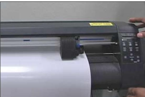
**3** Next load media into the cutter. Make sure to load the media with the colored side facing down and the white side facing up. After loading the film and setting the proper cutting conditions on your plotter, perform a test cut to make sure you have proper blade depth and a weedable graphic. For cutting Hotmark 70, we suggest a standard 45° blade at about 70 grams of force. After you have performed a satisfactory test cut, send the job from your sign making software.
